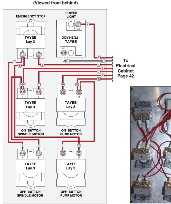
Figure 51. Control panel wiring.
